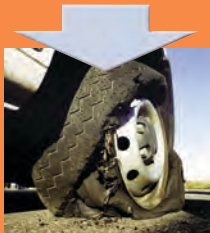
As a deflated tyre collapses, the wheel rim can come into contact with the road causing loss of control
