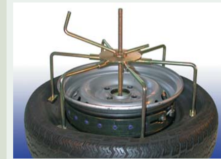
Tyron locks your tyre to the rim, forming a cushion of rubber so you can stay in control and drive to safety
